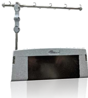
Figure 1: Photo of the IV pole collar installed on the Trima Accel IV pole.
