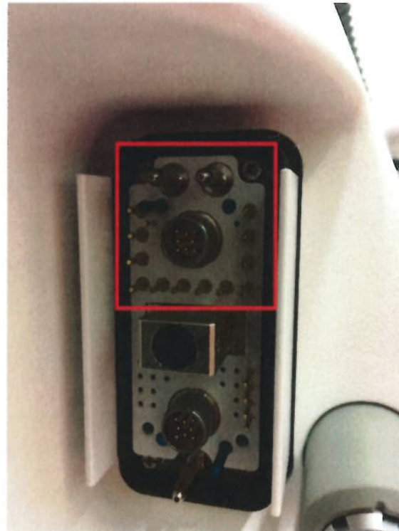
figure 2: example of X10 connector contact pin area which must not be touched
